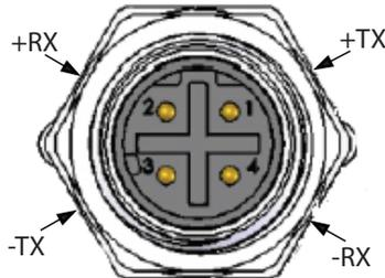
Figure 2: Ethernet Connector
